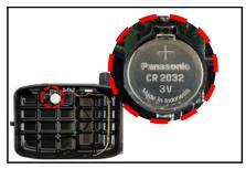
Ensure that remove an insulation film before install a battery.
