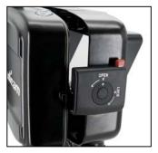
3. Close the housing while the housing lock is in the "Open" position.
