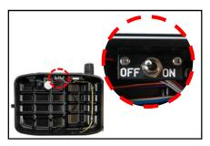
Switch the alarm on. The LED light will flash blue once and turn blue for five seconds indicating the battery is normal. Then it goes into flashing blue light standby mode.
