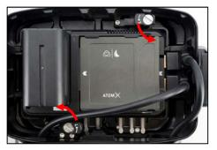
Before mounting the camera, connect HDMI 2.0 cables (IN and OUT) to the camera's HDMI connectors accordingly.
